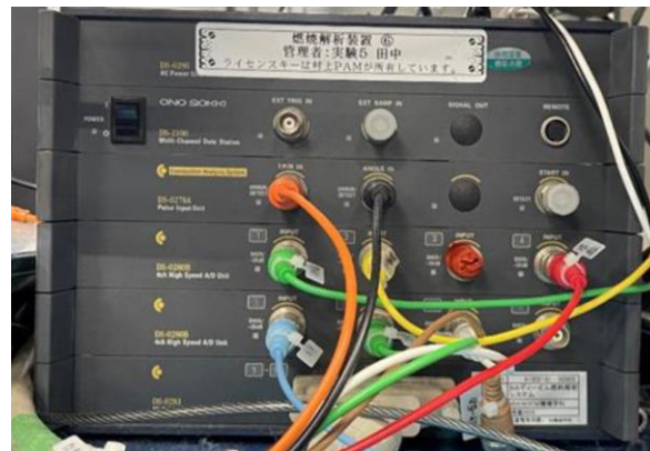
Fig.5.13 Exterior of Combustion Analyzer
