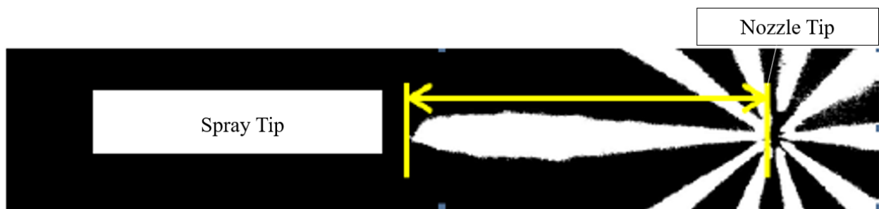
Fig. 4.6 Penetration Measurement Definition
