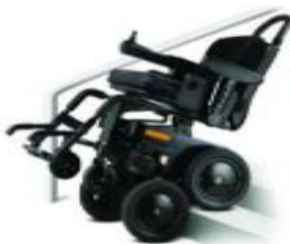
Fig. 1.4 A self-supporting powered wheelchair with a self-stabilizing device. (See <https://www.youtube.com/watch?app=desktop>)
