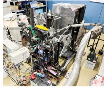
Fig.3 Engine on Evaluation Apparatus
