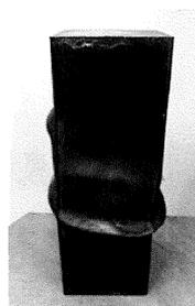
Photo.1 Failure mode of fiber reinforced square CFT
