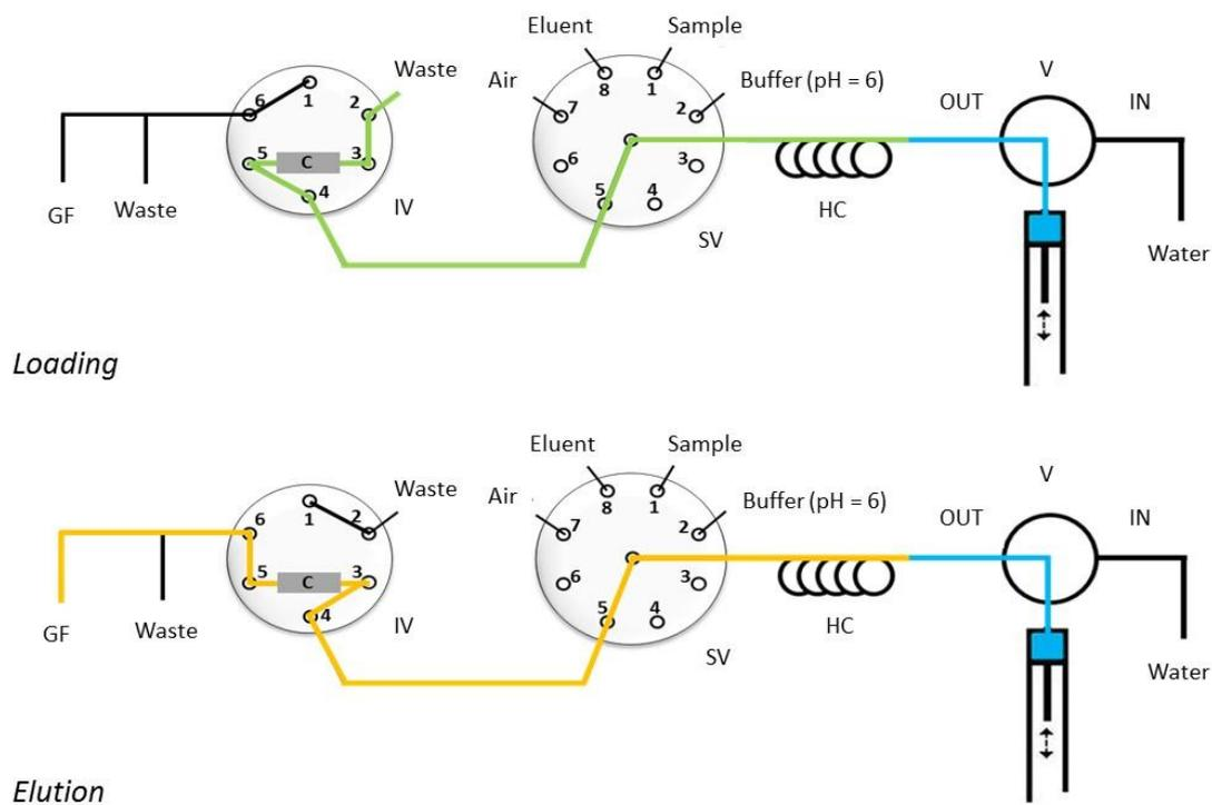
Fig. 6-1 Schematic diagram and the operation sequences (step 5: loading and step 11: elution) of the Auto-Pret-SI-SPE-ETAAS system for metal determination. IV, injection valve; SV, selection valve; V, valve; HC, holding coil; GF, graphite furnace; C, minicolumn packed with Nobias chelate PA-1.
