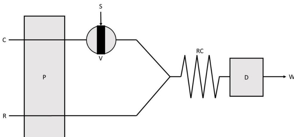
Fig. 1-1. The schematic diagram of a basic flow injection analysis system.
