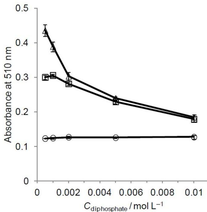
Fig. 3-6. Effect of diphosphate for vanadium determination
