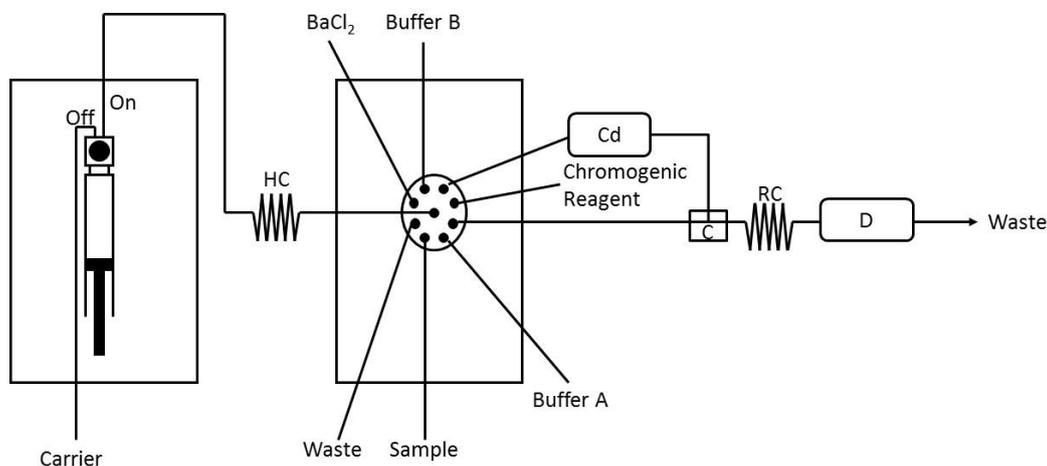
Fig. 2-1. SIA monitoring system proposed for  $\text{SO}_4^{2-}$ ,  $\text{NO}_2^-$  and  $\text{NO}_3^-$ .
