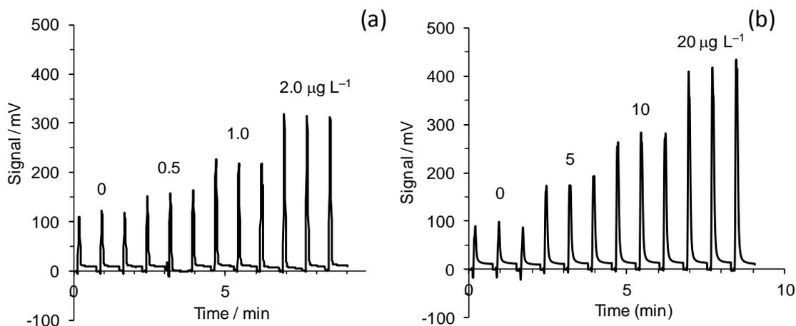
Fig. 3-7. Calibration sequences for vanadium and iron standards under the optimized conditions.
