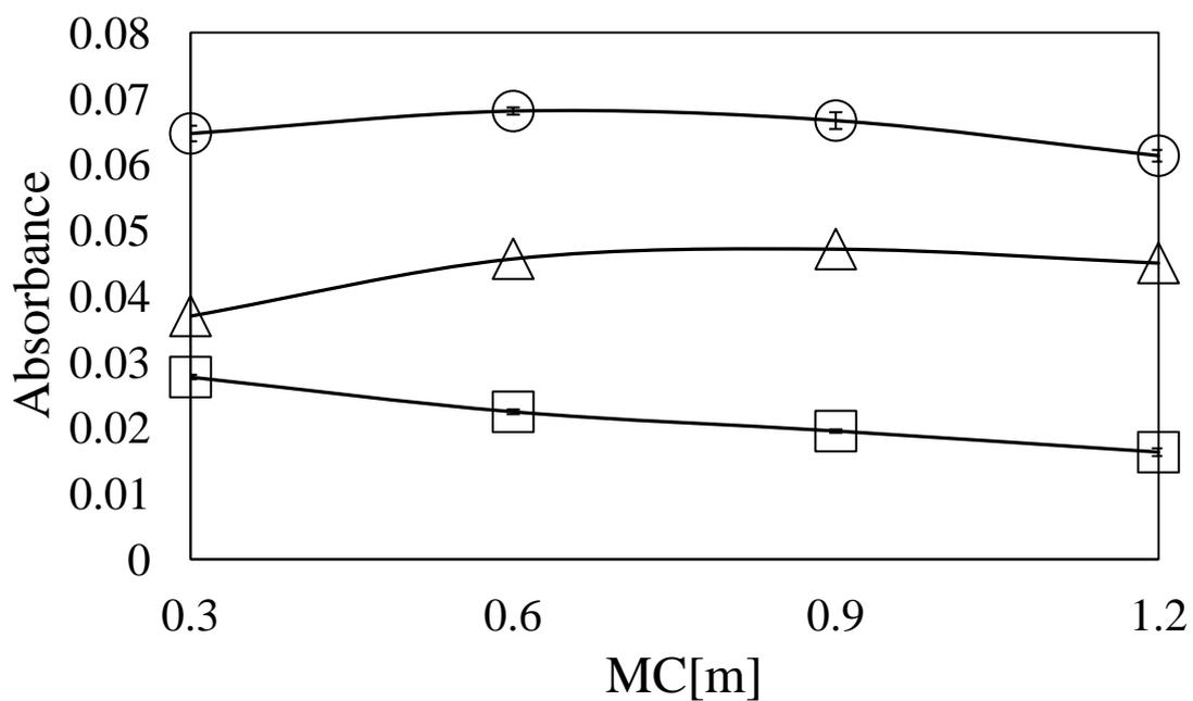
Fig. 4-2. Effect of mixing coil. ○: complex; △: net; □: blank
