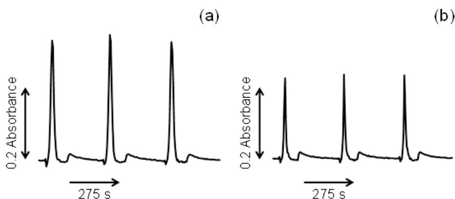
Fig. 5-2. Typical system outputs for (a) vanadium and (b) iron in certified reference material of river water (JSAC 0302-3b).
