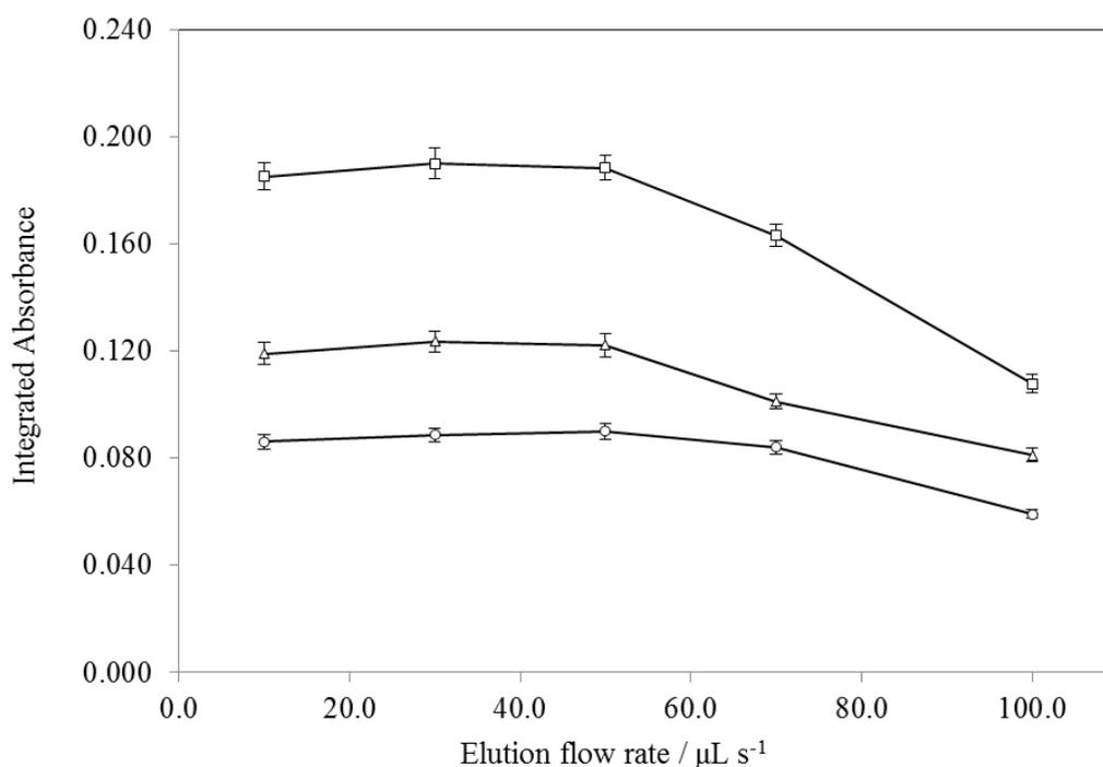
Fig. 6-3. Effects of the elution flow rate on the absorbance values of of  $2.0 \mu\text{g L}^{-1}$  V(V) ( $\Delta$ ),  $50.0 \text{ ng L}^{-1}$  Cd(II) ( $\square$ ) and of  $0.3 \mu\text{g L}^{-1}$  Pb(II) ( $\circ$ ). Volume of a loaded standard solution:  $3.0 \text{ mL}$ ; all other experimental parameters as in Table 6-2.
