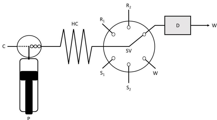
Fig. 1-2. The schematic diagram of a typical SIA system.
