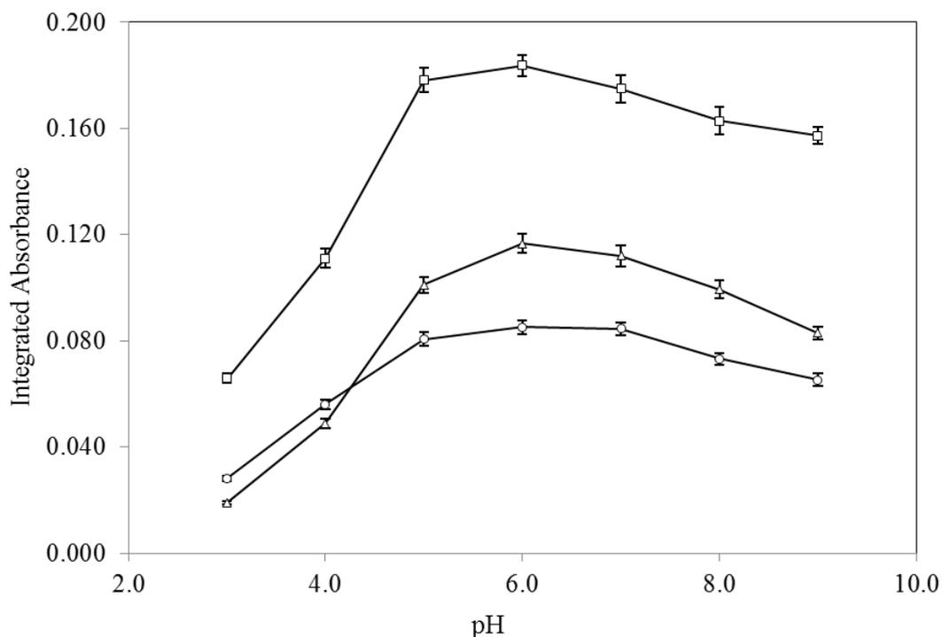
Fig. 6-2. Effects of the pH on the integrated absorbance values of  $2.0 \mu\text{g L}^{-1}$  V(V) ( $\Delta$ ),  $50.0 \text{ ng L}^{-1}$  Cd(II) ( $\square$ ) and of  $0.3 \mu\text{g L}^{-1}$  Pb(II) ( $\circ$ ). Volume of a loaded standard solution: 3.0 mL; all other experimental parameters as in Table 6-2.
