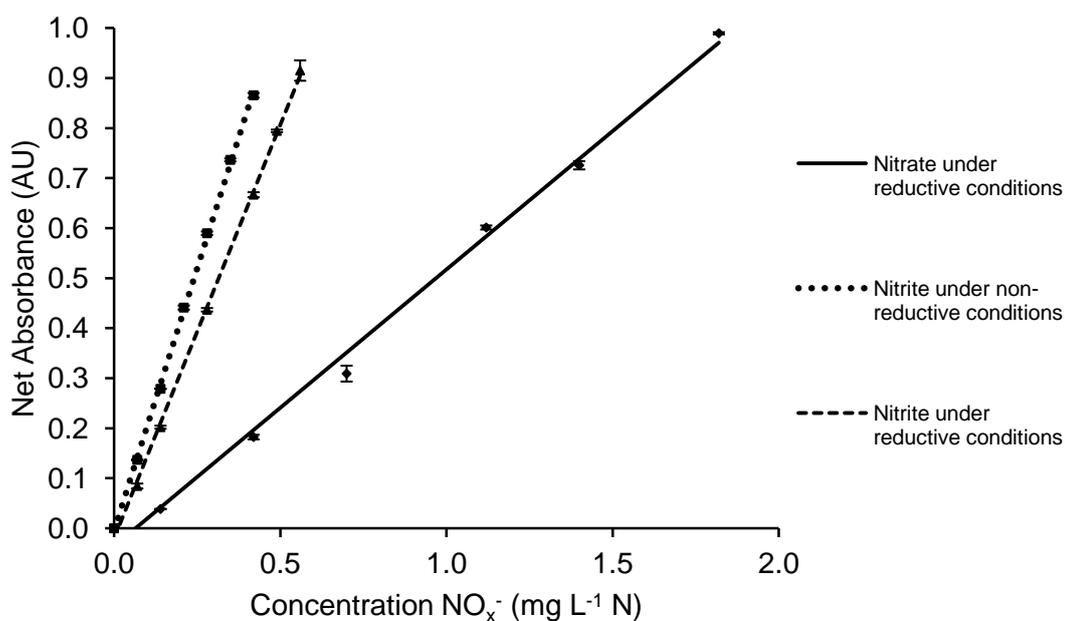
Fig. 2-3. Calibration graphs for nitrate under reductive conditions and nitrite under reductive and non-reductive conditions.
