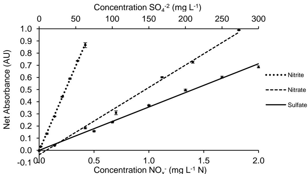
Fig. 2-2. Calibration graphs for sulfate, nitrite and nitrate.
