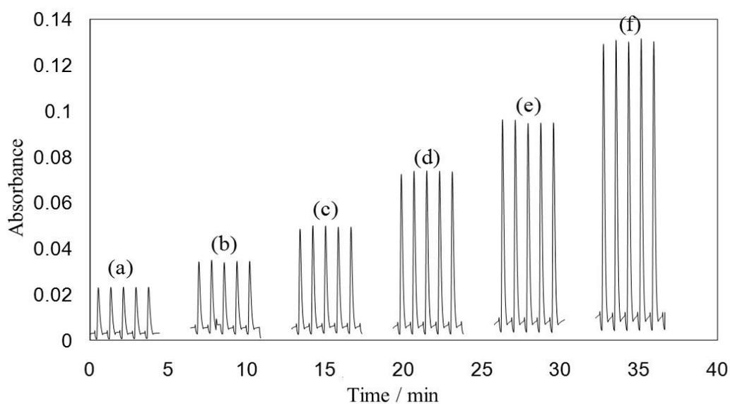
Fig. 4-6. System output response to standard palladium (II) concentrations in mg L<sup>-1</sup>. (a), 0; (b), 0.10; (c), 0.25; (d), 0.50; (e), 0.70; (f), 1.00.
